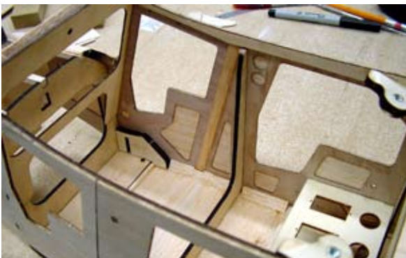
A look inside the cabin section showing the servo tray on the right and the landing gear mount on the left. The wing saddle doubler is at the top and the wing mounting bracket and blind nut are on the upper right.
