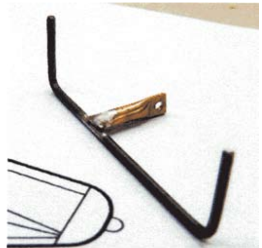
The elevator horn is silver soldered to the elevator linkage rod. The rod is 1/16" M.W and the horn is fabricated from 1/8" brass tubing.
