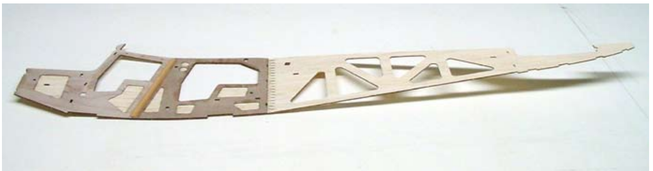
Here a completed fuselage side with doublers installed is ready for formers. Note the 1/32" balsa strip along the forward finger joint.
