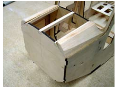
Forward section with corner sheeting installed and ready for shaping. Note that this model is being constructed with the glow firewall for use with a glow engine.
