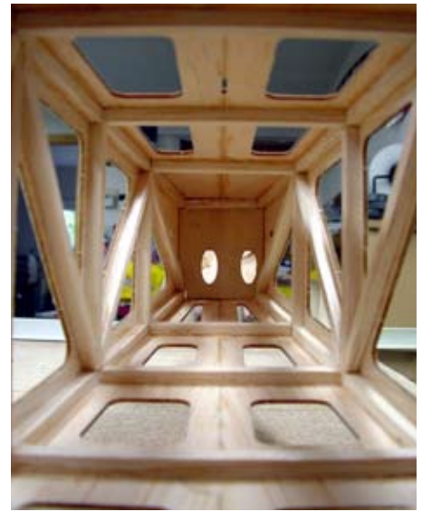
Looking back through the tail section of the model you can see the square balsa added to the fuselage sides as well as the top and bottom for additional strength.
