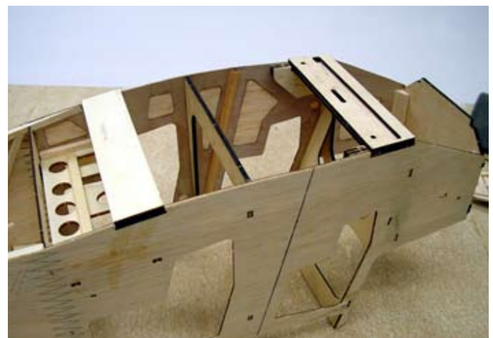
This view shows the cabin and forward section of the fuselage. The landing gear mount is on the right and the ply plate on the left is to support the aft mount for floats if so desired. A float kit is available for this model.
