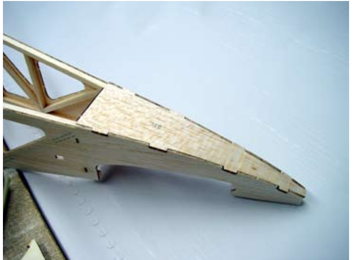
Bottom view of the tail section showing the bottom tail cap installed. The notch and tab construction assures that the fuselage sides are aligned and parallel to each other. No banana's here. Below this is the stabilizer saddle.
