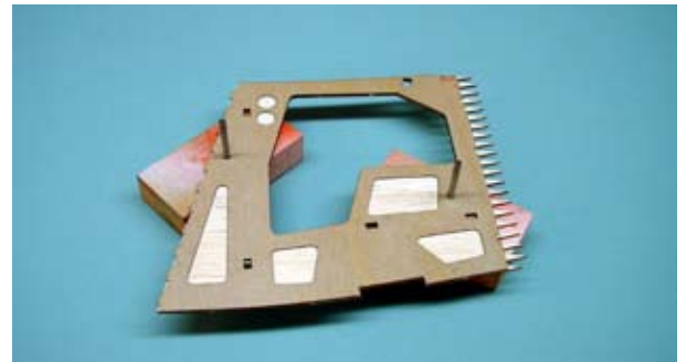
ABOVE RIGHT The center fuselage section shown here being assembled with the 1/64" ply doubler. The pinning method is used here to assure perfect alignment of all notches. Additional holes are provided to be used as glue ports. It is important that these ply doublers be positioned accurately.
