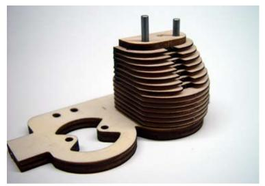
Now is a good time to glue this much of the assembly together. This can be done by running a liberal application of thin CA along the front and back of the cylinder from the inside. Be sure to hold the assembly compressed when applying the CA and avoid getting CA onto the registration pins. If necessary, use a clamp to compress the assembly until the CA has set.
