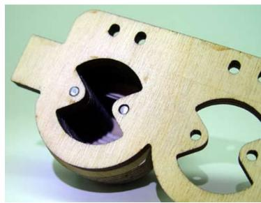
☐ 6 Install part #33 at this time. Due to minor variations in material thickness, it may be necessary to sand the top of #33 slightly so that it is perfectly flush with part #30.
