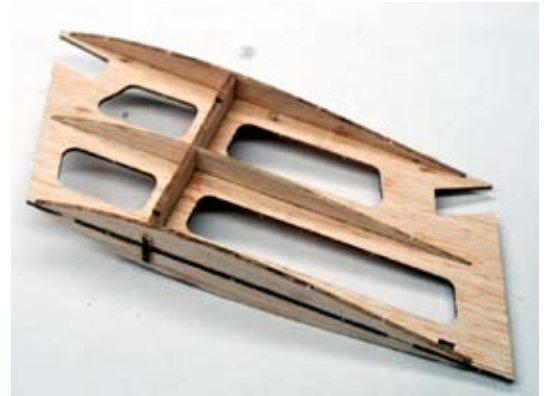
The pylon assembly under way. The ribs are split and tabs on the ribs fit into notches on the pylon core. The notches in the upper corners of the assembly will receive the rubber hooks.
