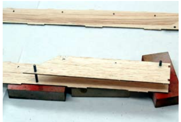
Both the fore and aft fuselage doublers are installed using pin registration to assure that all notches are correctly positioned. Take care to assure that the left and right side parts are correctly paired up as they are not interchangeable. 1.5° of left and down thrust is built into the firewall.
