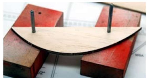
Laminating two WT pieces together to form the wing tip plate using the pin registration method.
