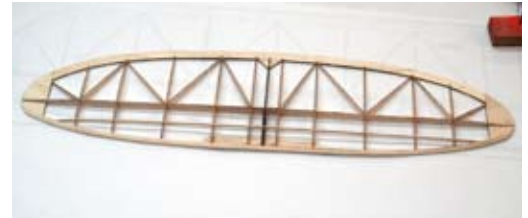
The completed stabilizer ready for sanding and covering.
