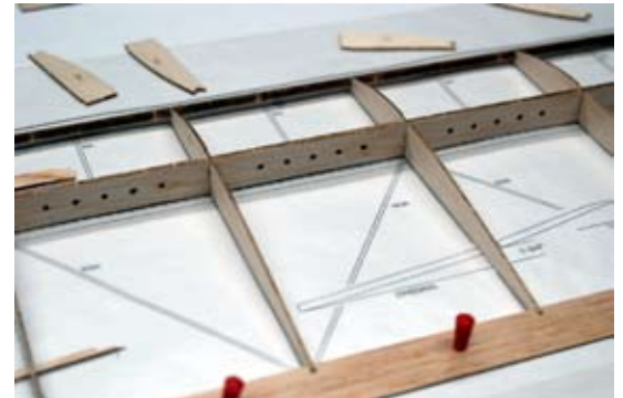
With all parallel ribs captive in the sheer webs, the trailing edges of the ribs are glued to the shaped trailing edge in the appropriate notches. The leading edge notches will engage the birds mouth at the front of each rib.
