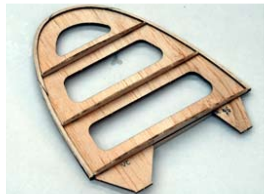
The completed vertical fin assembly. This assembly will plug into slots provided in the fuselage top and bottom for perfect alignment. Cover the fin before installing onto the fuselage.
