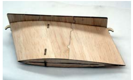
The nearly completed pylon assembly ready for covering. The rubber hooks slide into pockets in the pylon core after shaping the leading and trailing edges. The alignment tongue will slide into a notch in the bottom of the pylon and fit into a slot in the top of the fuselage for perfect alignment when installed.
