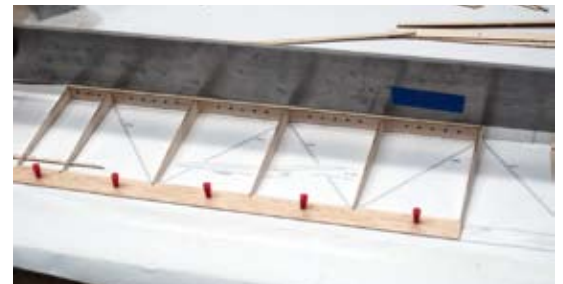
The top spar flange is installed using a heavy straight edge to assure good contact between the flange and the sheer webs. The holes in the back of the top sheer web will allow CA to be wicked into the sheer webs for additional strength.
