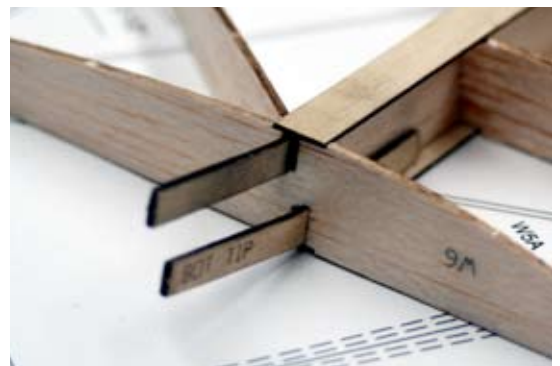
The wing panels are joined using these ply dihedral braces glued for and aft of the sheer webs.
