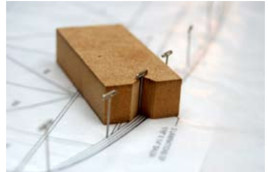
This simple guide will help keep the pins at 90° to the building board. A block with a V-notch cut into it will make the task easy.
