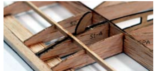
The stabilizer rubber hook shown here and the stabilizer alignment tongue (on the bottom) are permanently installed after sanding and covering the structure.
