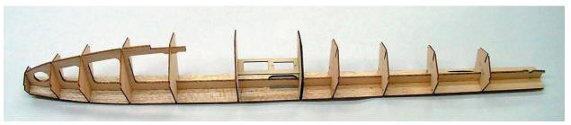
Install bulkheads B-1 through B11; note that B-6 and B-7 are designed so that the servo tray will orient correctly no matter which way they are installed. Be sure that B-7A is facing the aft end of the pontoon. Install the servo mount (SM) when installing the bulkheads.
