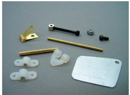
An effective water rudder can be assembled from these off the shelf components. The aluminum rudder and the brass flange will have to be fabricated from sheet stock. The flange will need to be soldered to the bottom of the tiller shaft. The rudder must remain loose and able to kick up to release any material that may strike it such as weeds etc. A plywood rudder is supplied and works just as well as the aluminum one shown here after water proofing with resin.
