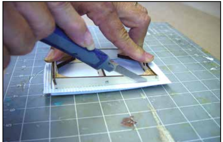
Trimming the hatch cover to the exact contour of the frame. If any plastic extends past the frame it can be sanded off.
