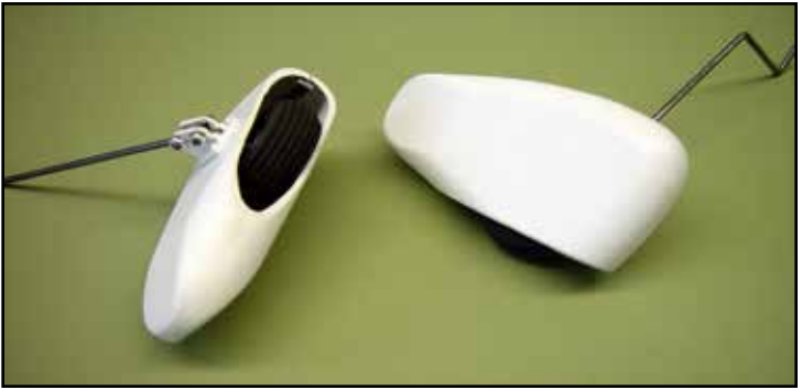
The completed wheel pants with the 1/8" wire gear installed. Trim the axle just shy of touching the opposite side of the wheel pant and install the axle support as shown. Two #2-56 x 1/2" bolts and NyLock nuts secure the mounting bracket to the gear leg.
