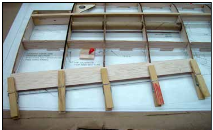
The top trailing edge sheeting (TTES) is secured with cloths pin until the aliphatic resin glue cures.
