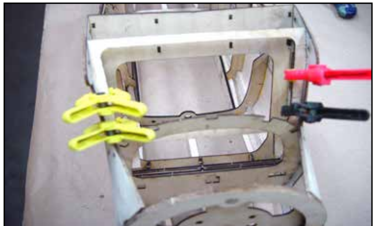
Installation of F2, use enough pressure to insure good contact with the fuselage sides. F2 should be flush with the top of the fuselage.
