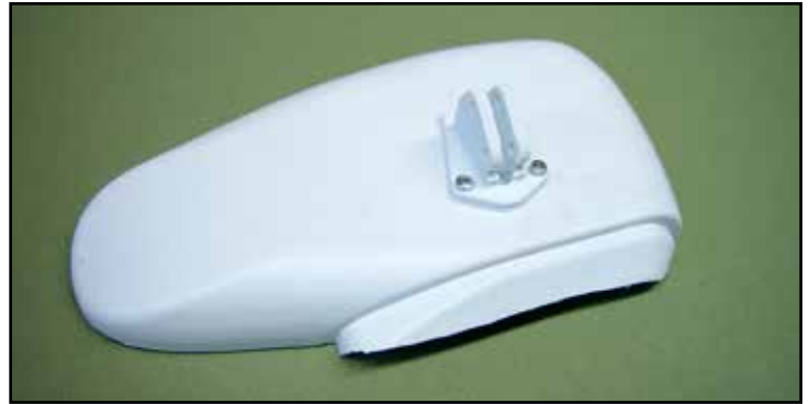
The wheel pant mounting bracket is attached with three #2 x 1/4" sheet metal screws and glue. Use the screw plate on the inside of the part.
