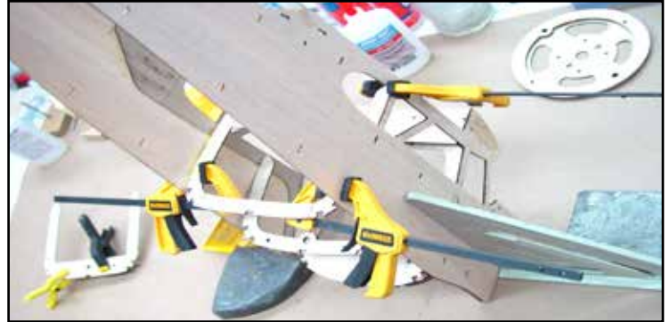
Clamps secure F5 firmly to the fuselage sides as the Epoxy cures. A square is used to insure the sides are square to each other.
