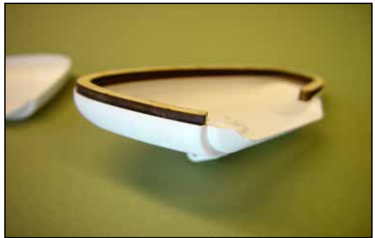
WPJ is installed half way into one of the wheel pant shells with Pacer Formula 560 Canopy Glue.
