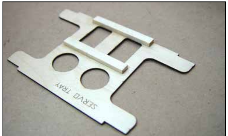
To supply thread grip, two 1/4" x 1/8" basswood sticks are added as screw rails to the servo tray.
