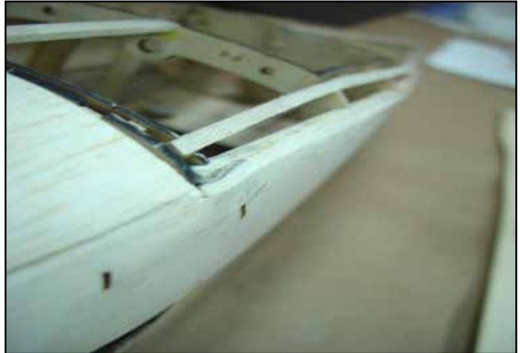
Sand a bevel into the corners in preparation for installing the corner sheeting.
