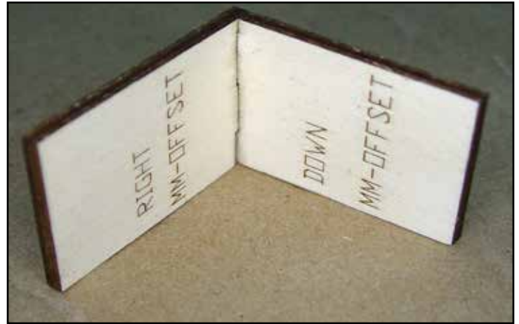
The assembled motor mount offset jig. Be sure to orient it correctly when assembling your motor mount.
