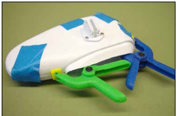
The wheel pant halves are secured with masking tape and two clamps are used to insure that WPJ is in good contact with both halves at the opening. A liberal bead of glue is added to the entire length of WPJ to complete the assembly.
