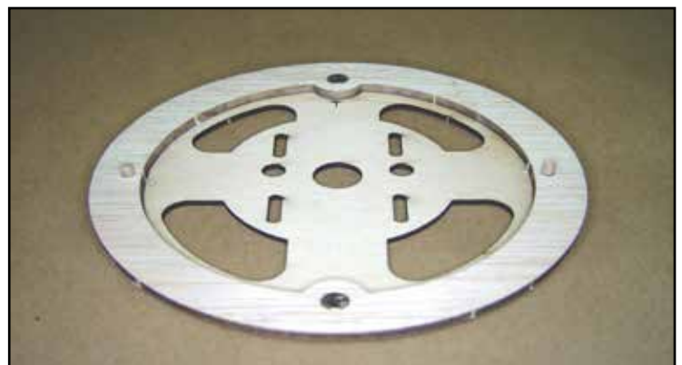
The firewall (F1) sub-assembly showing the F1-A in place and two magnets installed. The dowels will center the cowl and the magnets will retain it. The slotted holes will allow for vertical adjustment of the motor mount for centering in the cowl.
