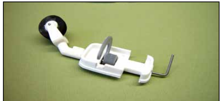
Rudder bearing assembly ready for installation onto F12.
