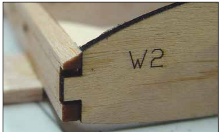
In preparation for installing the leading edge sheeting, FLE is tapered to contour with the ribs.
