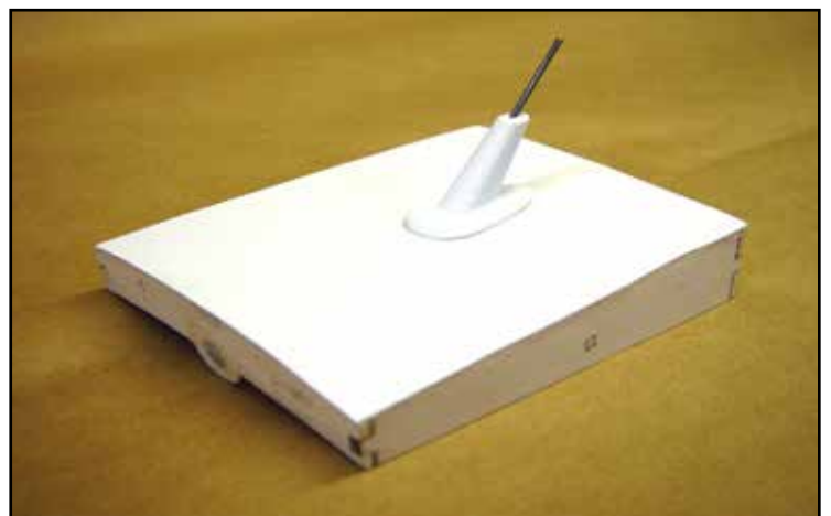
The completed battery hatch with the simulated VHF antenna as the hatch handle. The hatch is retained by the magnets fore and aft in the frame.
