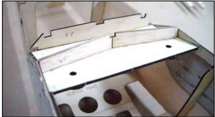
WMP installed with WF and ready to install FCB parts in the corners. The FCB parts will allow carving these corners smoothly into contour with the aft fuselage top.
