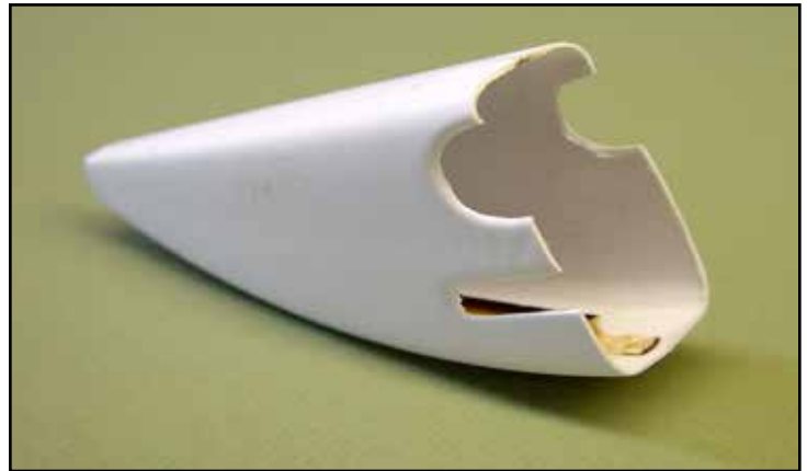
Tail cone halves have been trimmed and assembled with TCJ. Rudder horn opening and elevator joiner openings have been cleared of material.
